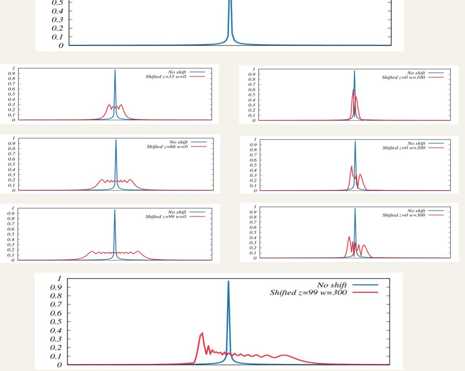
The smearing in the case of the 'jerk' search depends on two quantities z and w. These represent the first and second derivative of the pulsars frequency. Top: Signal from a stationary pulsar. Middle: The red line shows the smearing for different values of the first derivation (middle left) and second
