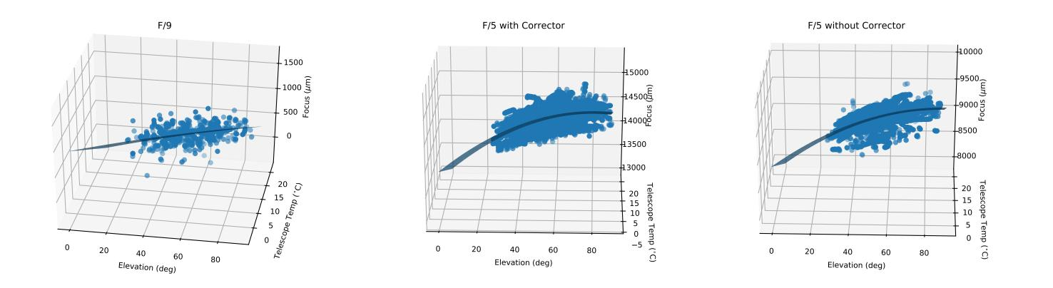
The RMS scatter is 130-160 microns in each case. Only the focus axis is shown here, but similar behavior is seen for the other axes of secondary mirror motion. Fitting the models to data from 2017-2018 and checking against data from 2019 yields similar results, but slightly worse scatter, 140-180 microns.
