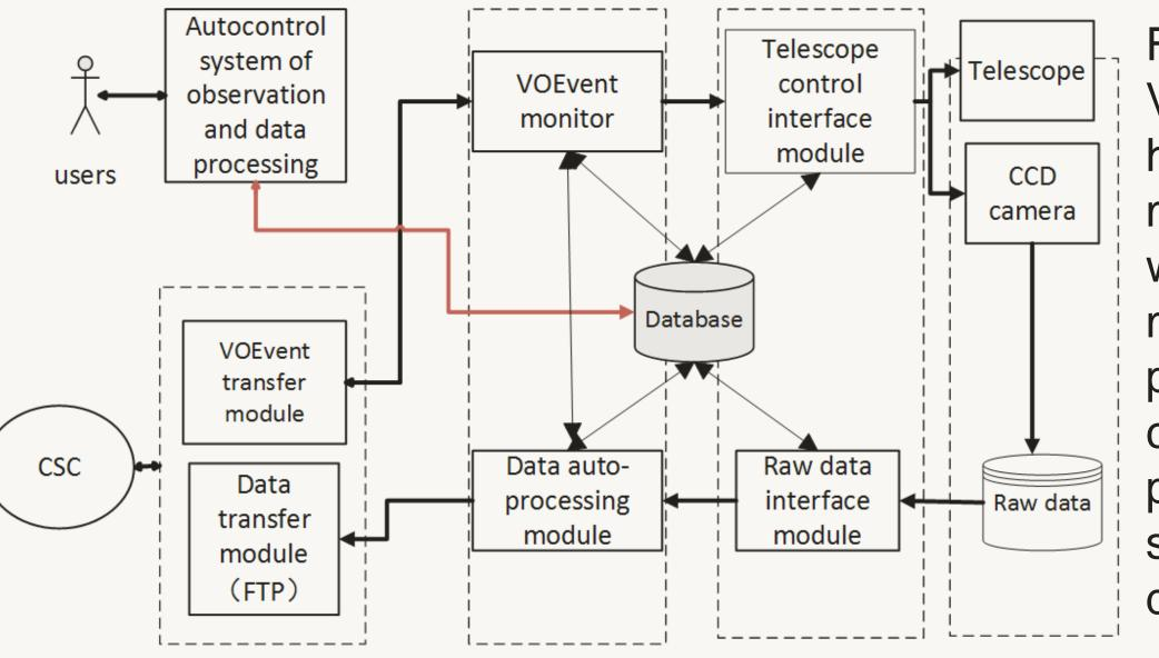
For the interface to CSC, **VOEvent module** handles the alert messaging with CSC, while data transfer module uploads data products, data file checksum, and processing log to its FTP server for CSC to download and archive.
