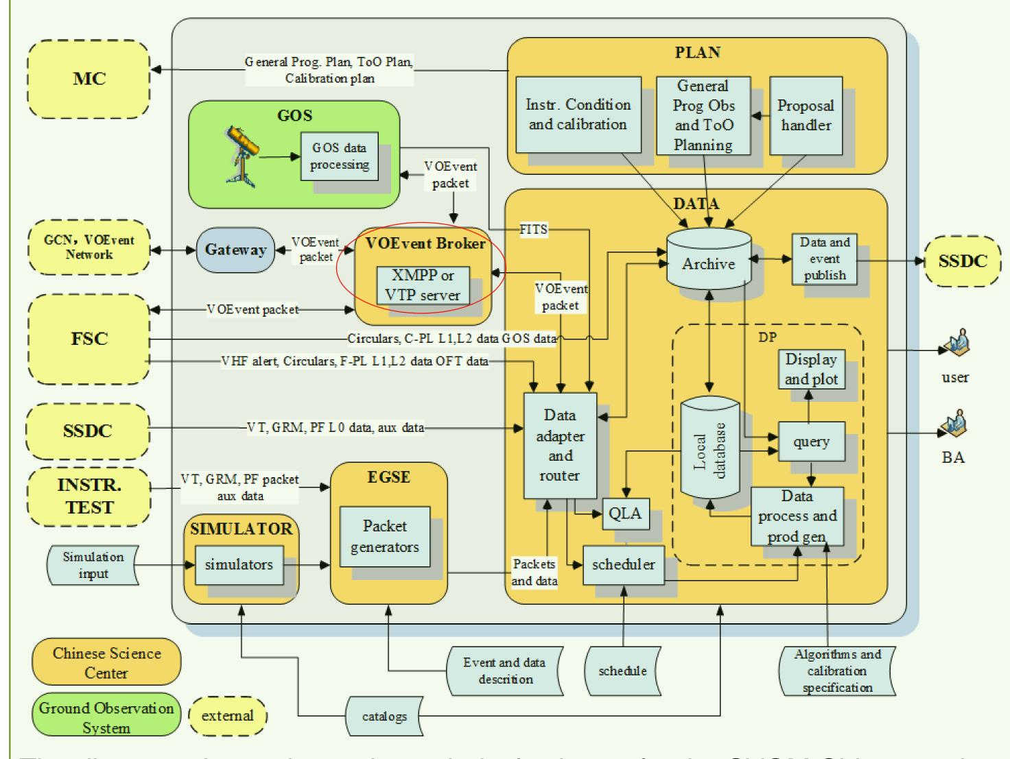
The diagram above shows the technical scheme for the SVOM Chinese science application system. It contains a lot of modules and have complicate logistics, note is the ground alert distribution subsystem showing within the red circle, that is the VOEvent broker, which is an interface between Data reduction subsystem and the global VOEvent network and French Science Center.
