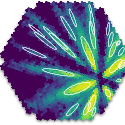
**a example of raw data from CTA:** this is the sum of time-integrated ages (over a window of *20 ns*) of the Cherenkov light from a single imma-ray induced air-shower, as seen from multiple telescopes. The **igin of the photon** is at the point where the axes of the ellipses cross. The **energy** is proportional to the light collected. In normal data taking, ese images are recorded (with time information) at a rates around 10KHz
