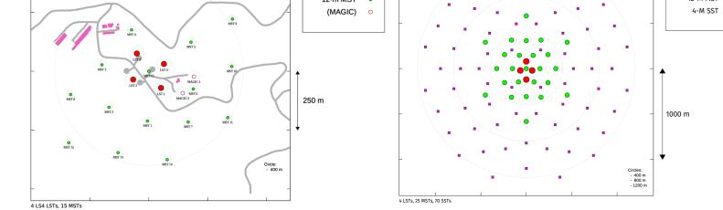
CTA Observatory full array configuration**: 118 telescopes, 3 telescope classes** (large LST, medium MST, and small SST) , operating on **2 array sites**
